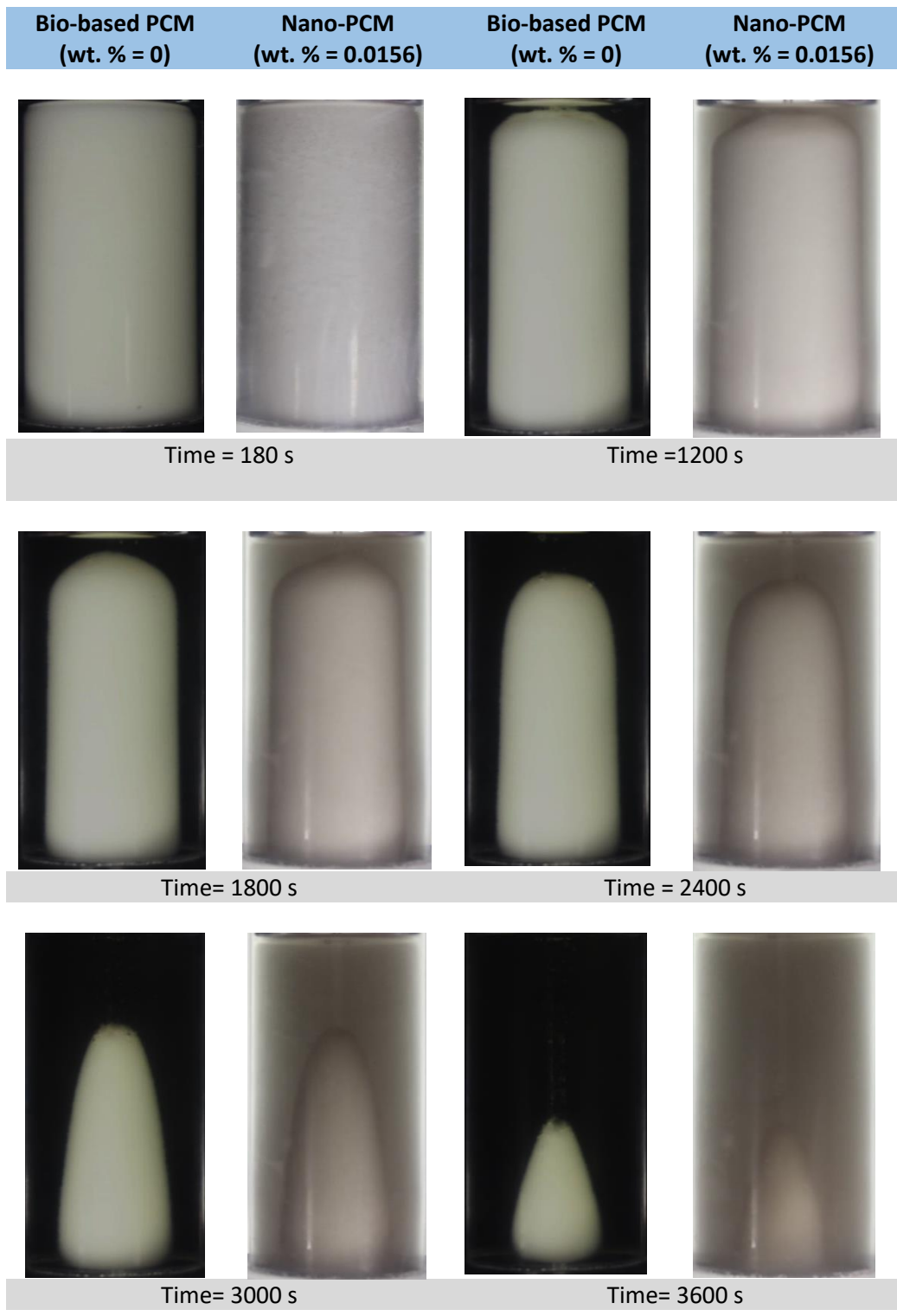
Fig.7. Visualization comparison between bio-based PCM (wt.%=0) and 0.0156 wt.% nano- PCM, H=10 cm.
